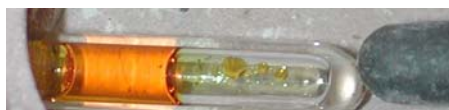
Melted NbCl_5 at 210°C in high temperature cell (20-250°C) for in situ Raman spectra measurements
